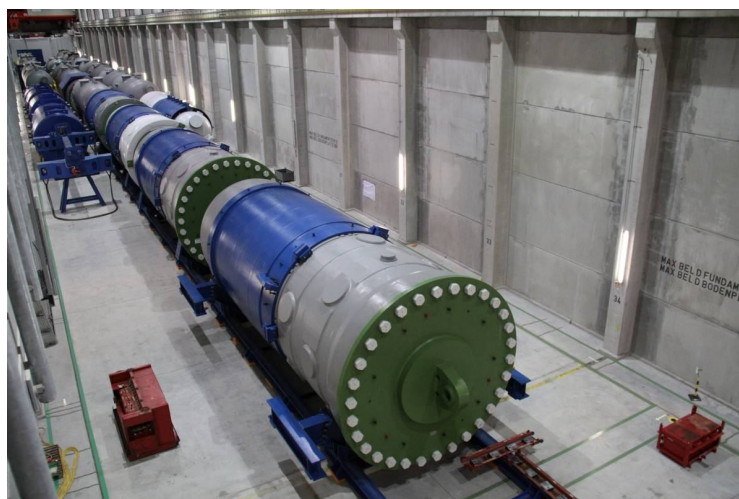
Fig. 1.6.1.3 -5 Storage hall for RPVs
