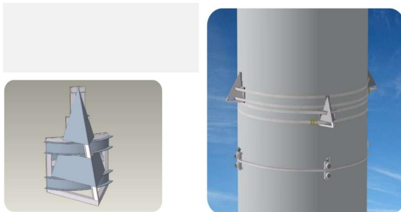
Installation of ice deflectors
